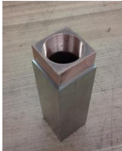
Figure 4. Completed thermal fatigue specimen with 0.100” thick H13 on C1100 copper.
