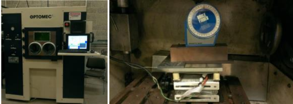
Figure 3. Northern Illinois University LENS™ machine (left) and heated work table with copper substrate mounted in the chamber (right).
