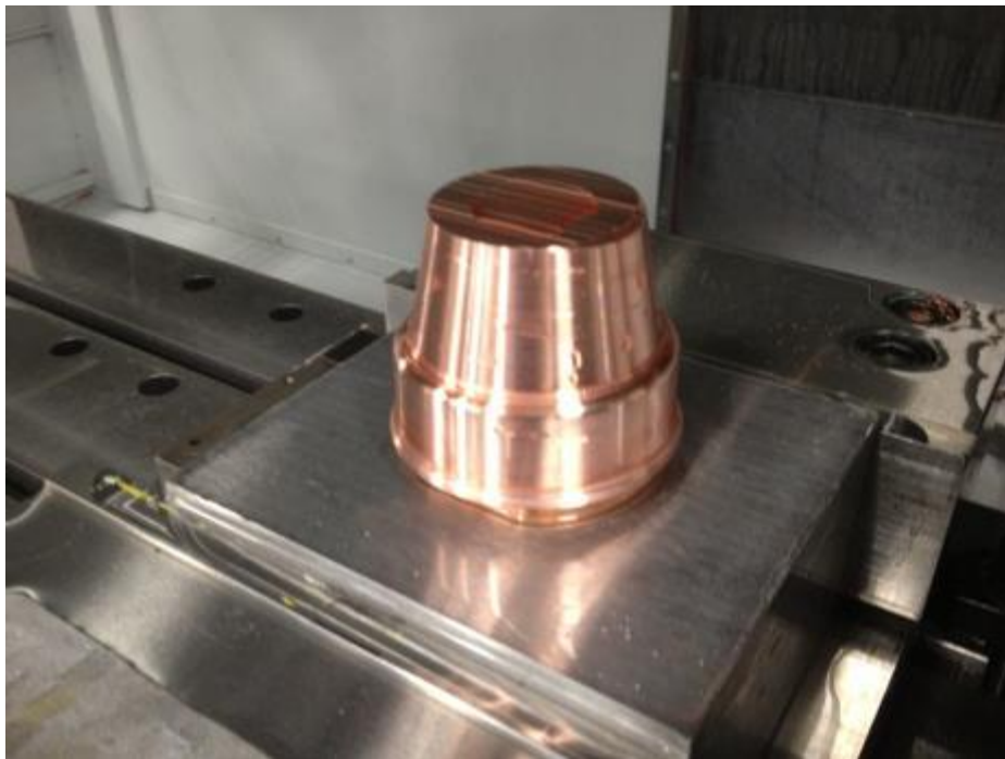
Figure 18. Machined copper substrate for Shiloh commercial core on the heated table in the LENS TM machine at NIU.
