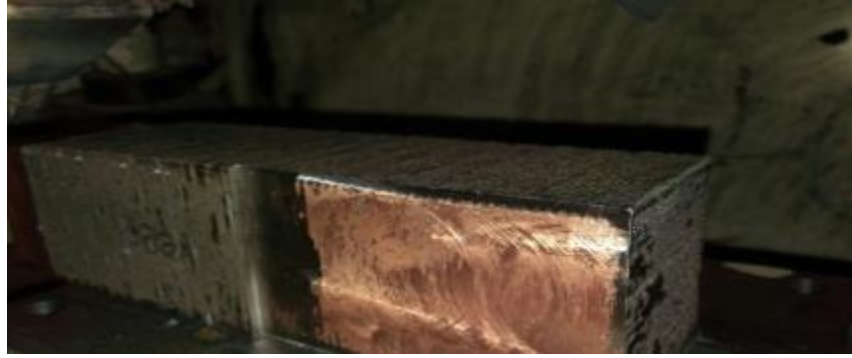
Figure 13. Cracked region machined back down to copper for re-deposition.
