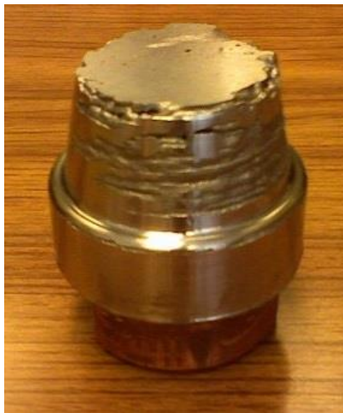
Figure 20. Commercial core subsequent to LENS TM deposition with H13 and rough machining at Mo-Tech.
