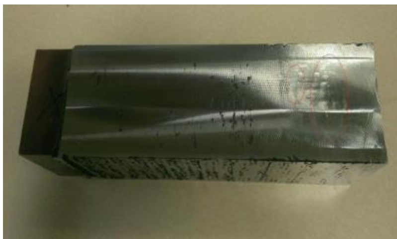
Figure 12. Circled in red are the cracks formed during deposition from the focusing lens melting.
