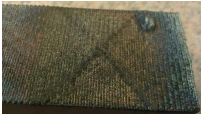
Figure 14. “Sawtooth” pattern formed on second layer of H13 deposition.
