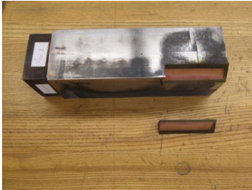
Figure 15. Thermal fatigue specimen with the sides 1-4 corner removed via wire EDM.
