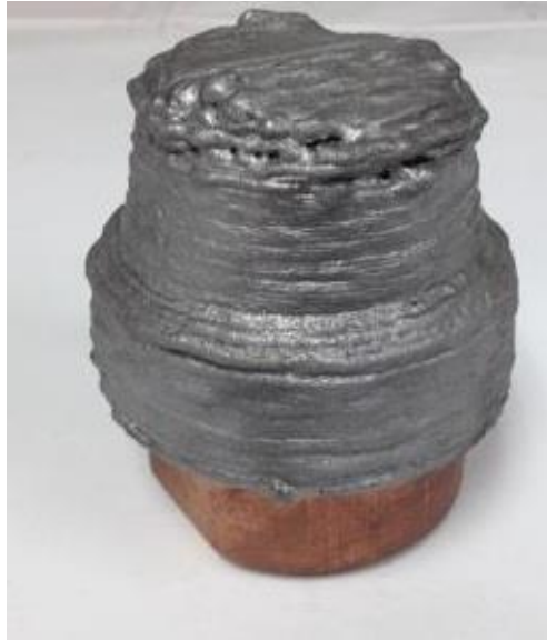
Figure 19. Commercial core subsequent to LENS TM deposition with H13.
