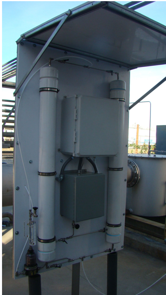
Figure 5 Biogas Analyzer Installed in ABI Plant (Feb., 2012)
