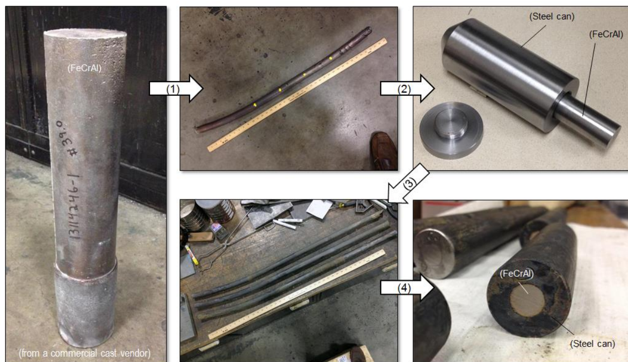
Figure 7. Hot-extrusion process of the C35MN5 alloy to make 10mm-diameter bar samples.
