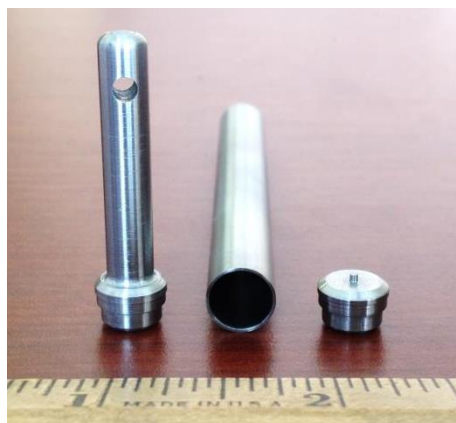
Figure 9. Machined tube and end caps for ATF-1 irradiation campaign.
