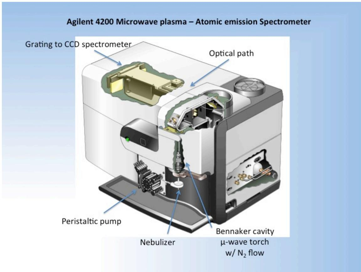
With this device, we can now quickly assay the detailed cold metal load in of our outbound Cu-64 and Zr-89, correlating this part-per-billion broad-element analysis with our effective specific activity measurements made by chelator titration.
