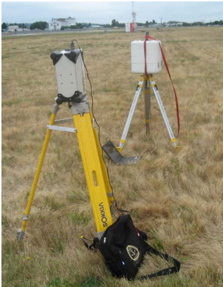
Figure 8. Pressurized ion chamber and high-purity germanium detector set up for measurements on a calibration line.
