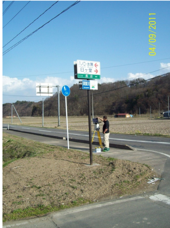
Figure 4. A member of the ground team performs ground truth measurements with an HPGe detector in Japan.
