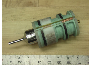
Figure 4. HEML projectile with tool hardened tip
