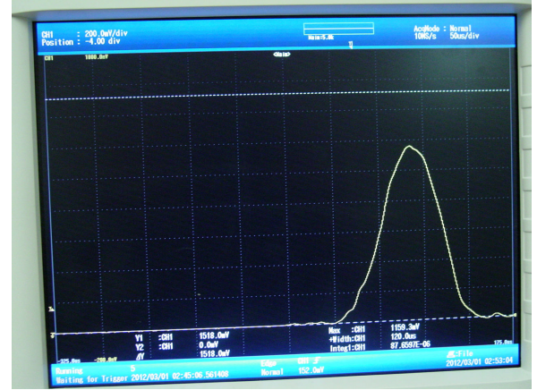
Figure 9. Calibration shock pulse (acceleration vs. time)
