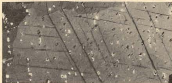
Fig. 14a-c — Comparison of x-ray diffraction structures and microstructures before and after cycling of rods shown in Fig. 6a. Photomicrographs under polarized light at 150 \times . X-ray photograms 2 \times .
