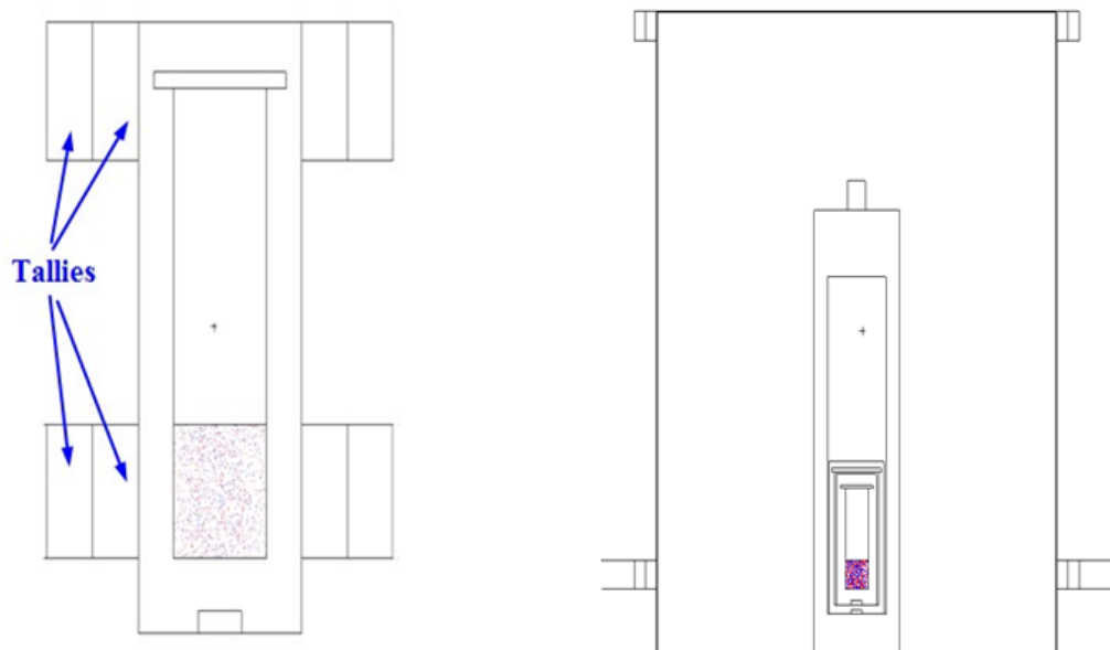
Figure 2. Shipping configuration with inner & middle containers, source capsule, and drum.
