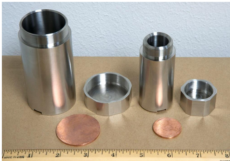
Figure 1. Photo of LANL prototype “middle” and “inner” containers with lids removed.
