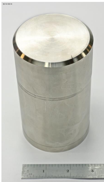
Figure 5. Nested & Sealed “middle” and “inner” containers
