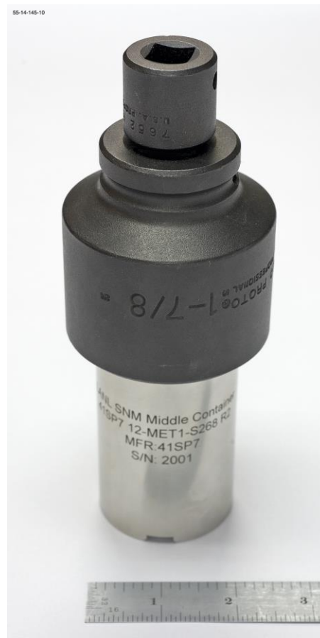
Figure 7 (left). Jig/Pig holder for middle container. Used as shield/fixture for sealing Figure 8 (right). Middle container with socket driver used to seal
