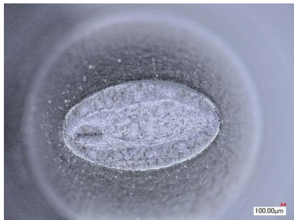
Fig. 40. Fracture surface for expanded longitudinal tensile test specimen.
