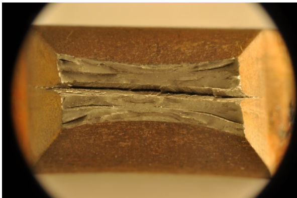
Fig. 50. Top view of fracture surface for expanded and strain-aged longitudinal tensile test specimen 90° from weld seam.
