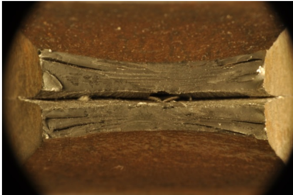
Fig. 48. Top view of fracture surface for expanded longitudinal tensile test specimen.
