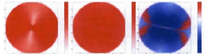
Figure 4. ODD Kernels trained to preserve smooth contours against background clutter. (a) Co-occurrence matrix obtained from all pairs of edges belonging to 10,000 target objects. (b) Co-occurrence matrix for edge pairs belonging to background clutter. (c) ODD kernel computed from the normalized difference between target and background co-occurrence matrices.
