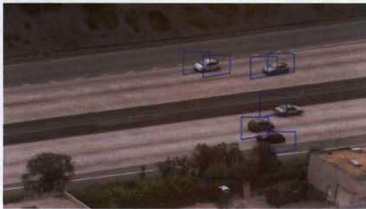
Figure 9. Example output. Every car has a detection on it with one false positive. Although this is a very desirable outcome, it did not score well due to the false positive.
