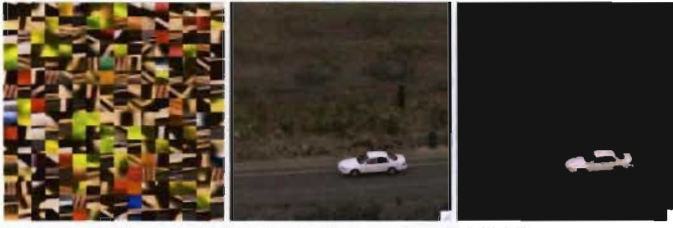
Figure 1. From left to right: (a) Learned over-complete color/texture dictionary for the helicopter dataset. Our dictionary captures orientation edge structures and non-oriented color features. (b) Example image patch from a training sequence. (c) Reconstruction of image patch using local sparse representations over the learned dictionary.
