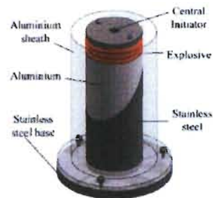
Figure 2. The Fils experiment. The aluminum (top) and stainless steel (bottom) components were machined to a surface roughness of \lambda/2 \mu\text{m} and were flat such that the maximum gap that could exist between the sliding surfaces was \leq 25 \mu\text{m} . The components were held in contact by gravity.
