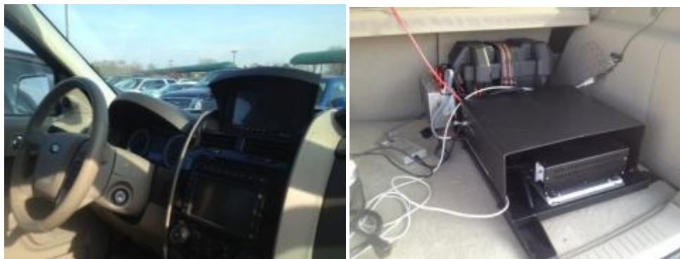
Figure 101 - Installation of the rapid prototyping system in the vehicle.
