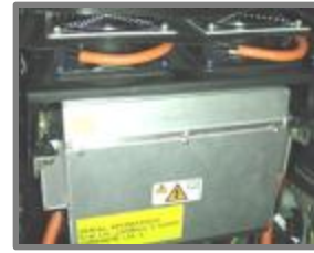
Figure 6: 1.4 kW Charger with Revised Cooling Fans
