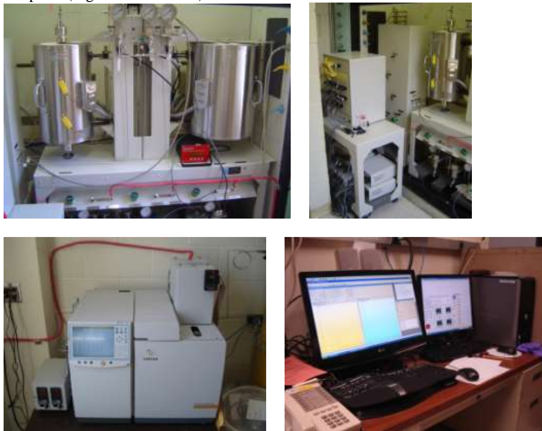
Figure 3.1 High pressure and temperature flow reactor system
