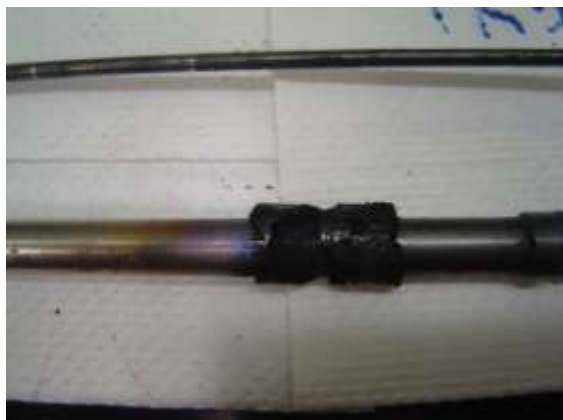
Photo 6.1. 6.5” spool with carbon “ring” after reaction (exp. TR-51)
