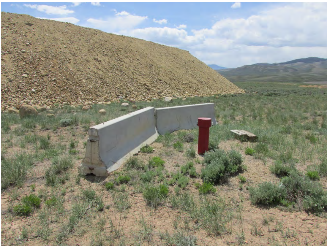
GUD 6/2013. PL-6. Monitoring well 0716 protected by concrete barriers.
