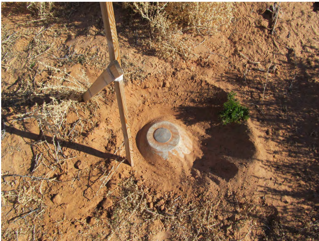
TUB 4/2013. PL-3. Benchmark No. 1 southeast corner.
