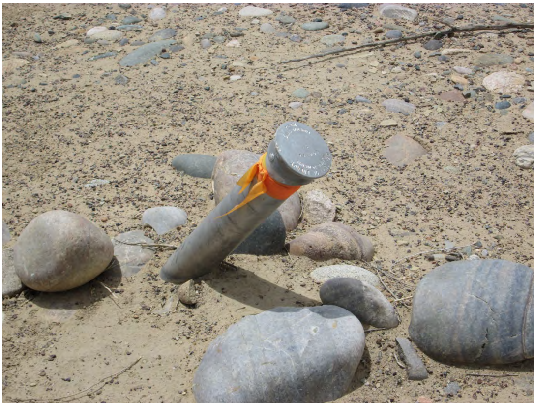
SHP 5/2013. PL-9. Erosion marker ECM-5A, bent but functional.
