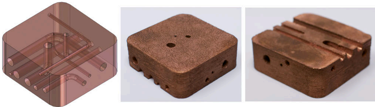
Figure 9: 3D CAD model of the cooling channel test block (CCTB) showing internal cooling channel geometry (Left), and photographs of the sectioned EBMed CCTB showing cooling channels of 1.5mm, 4mm, and 7mm in diameter.
