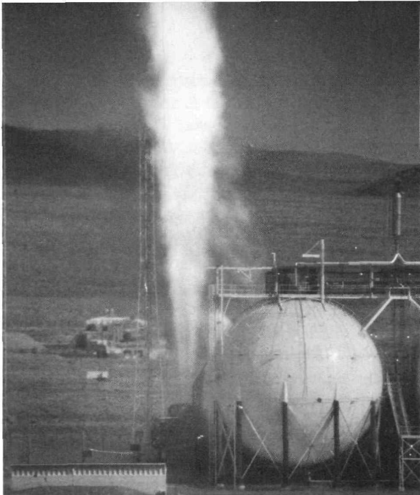
Exhaust blast from a successful reactor test shoots high in the air over the test cell propellant tanks. (Telescopic lens photo.)
