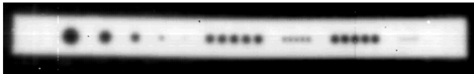
Figure 2. Flat panel neutron image of a 0.5mm thick cadmium test piece. Hole sizes include single hole diameters of 2, 1.5, 1, 0.5 and 0.25mm and groups of holes, as follows: 1mm dia., with 0.5mm spaces, 0.5mm dia., with 0.5mm spaces, 1mm dia., with 0.25mm spaces, and 0.25mm dia., with 0.25mm spaces. Hole separations of 0.25mm are detected, representing a spatial resolution of 2 lp/mm.
