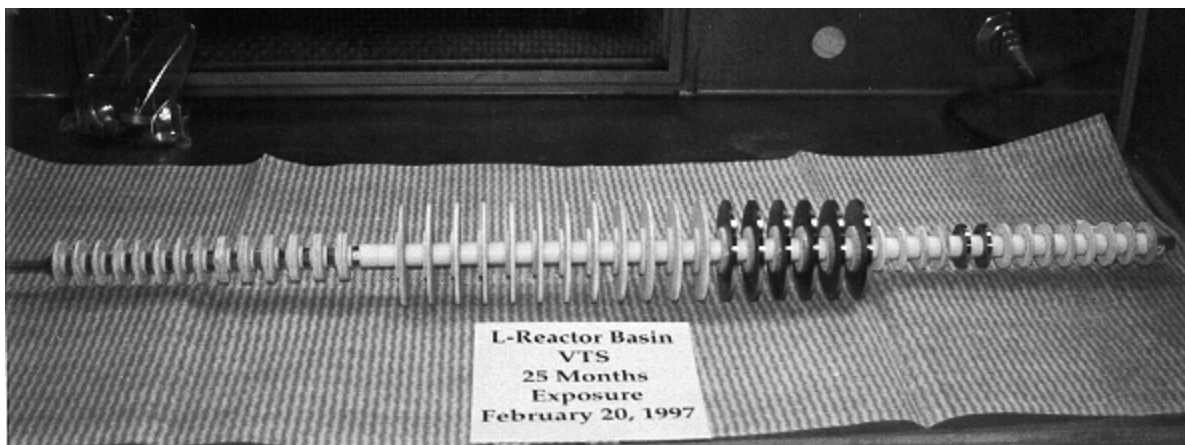
Figure 4. Typical Corrosion Surveillance Rack
