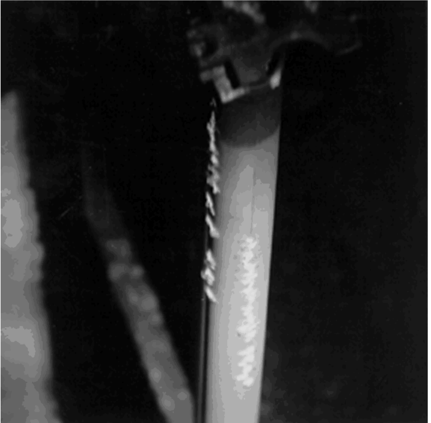
Figure 2. Nodular Corrosion Product on Underwater stored Mk 22 Fuel Assemblies
