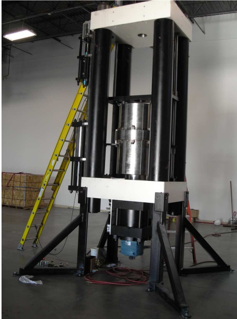
Figure 8 Picture Showing Construction of UDS (Main Test Vessel, Hydraulic Charge Pump, and Hydraulic Circulation Pump have been added)
