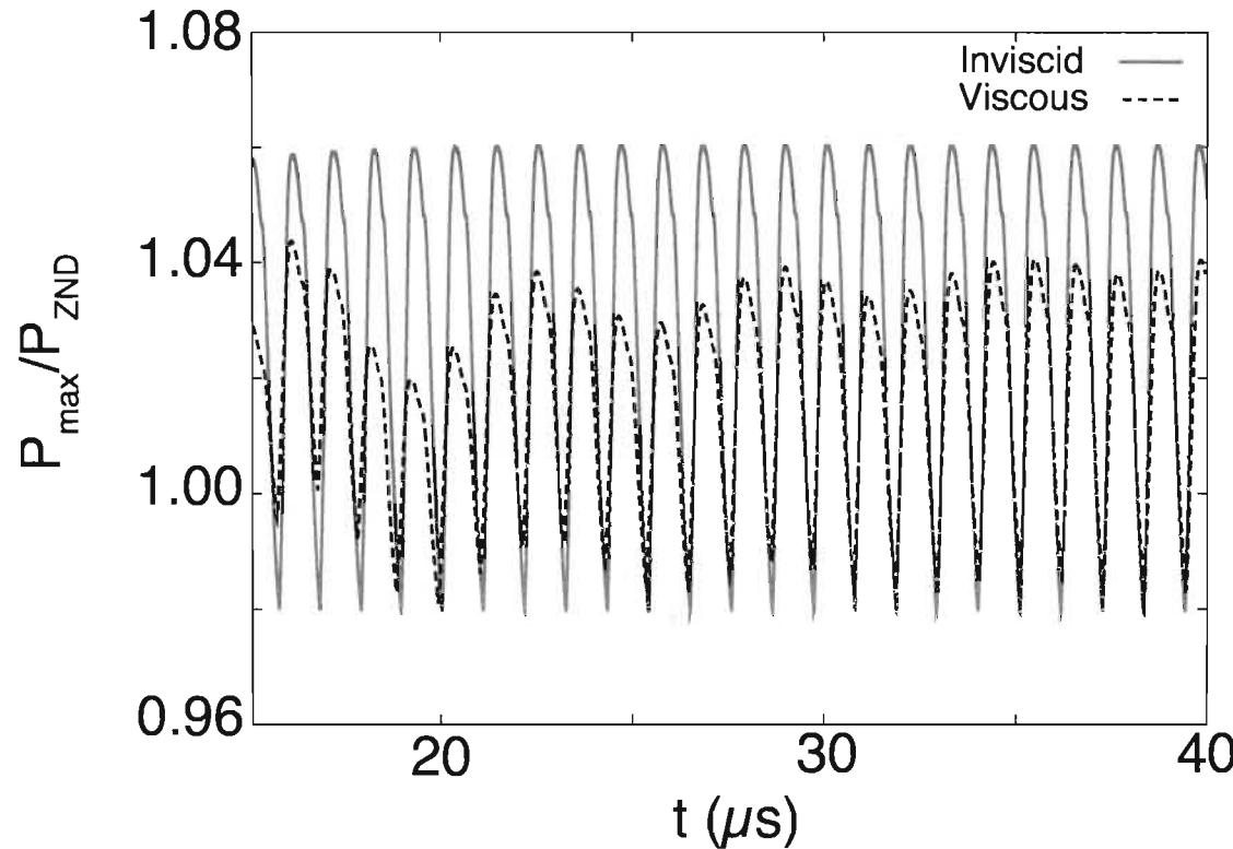
The addition of viscous effects have a stabilizing effect, decreasing the amplitude of the oscillations by  $\sim 25\%$ .
