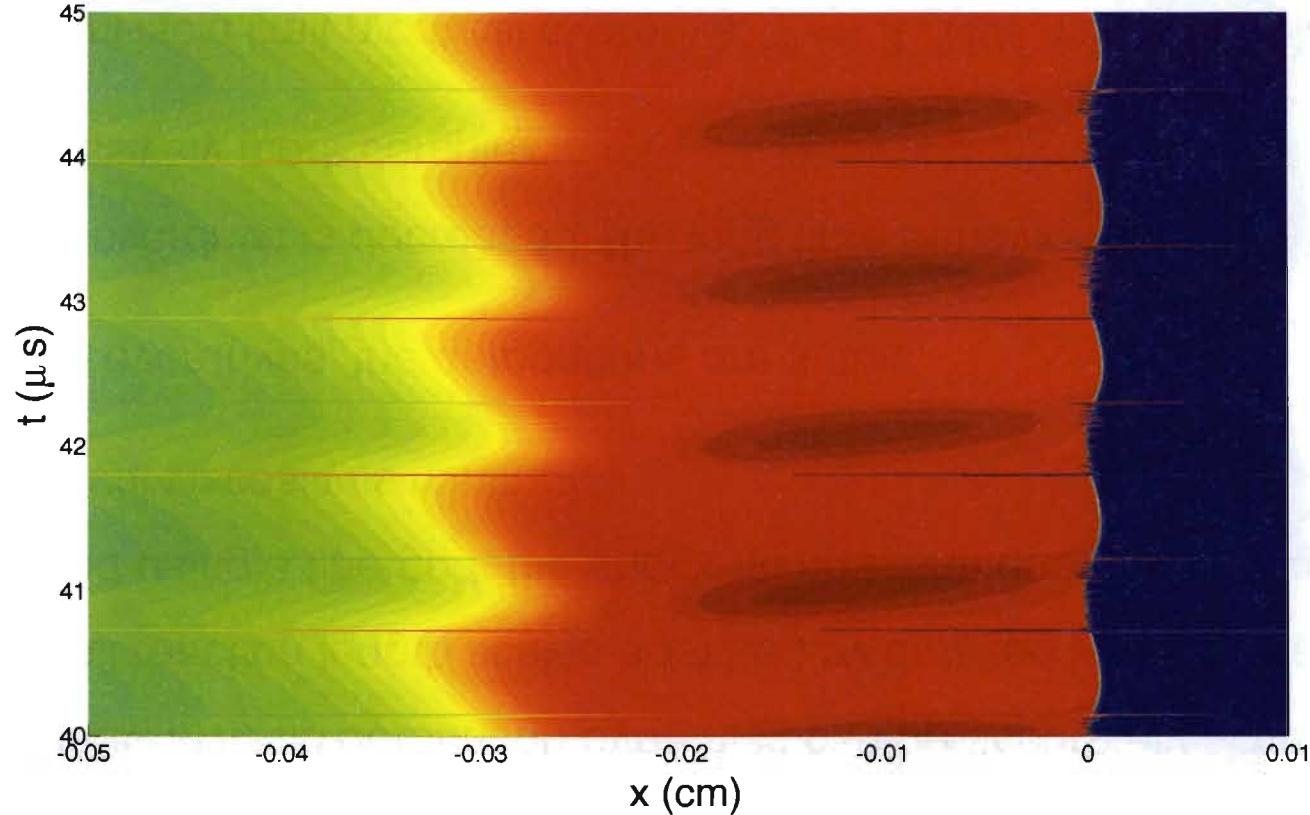
A  $x$ - $t$  diagram of density in a Galilean reference frame traveling at 2057  $m/s$ .
