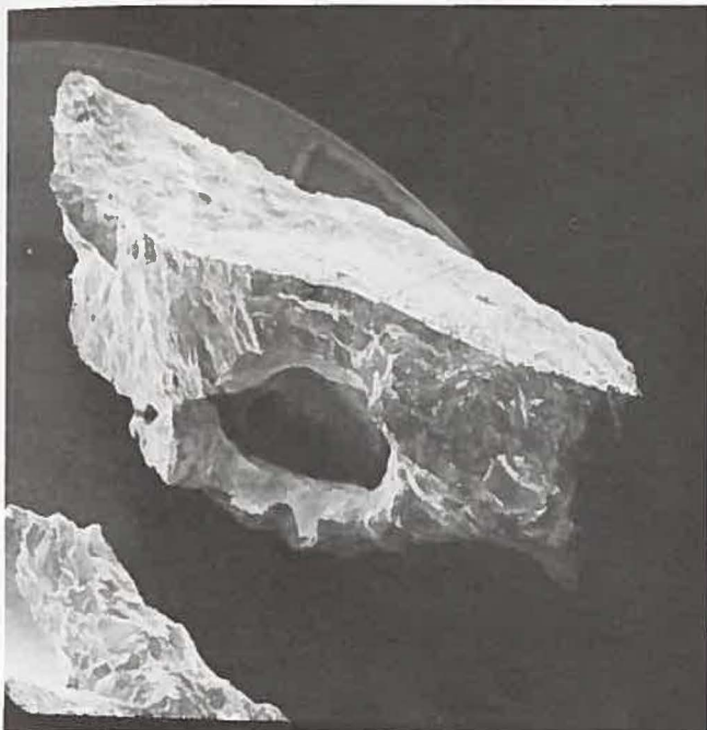
Fig. 52(a). Fuel Particle with Central Void Surface. Neg. No. MSD-200550.
