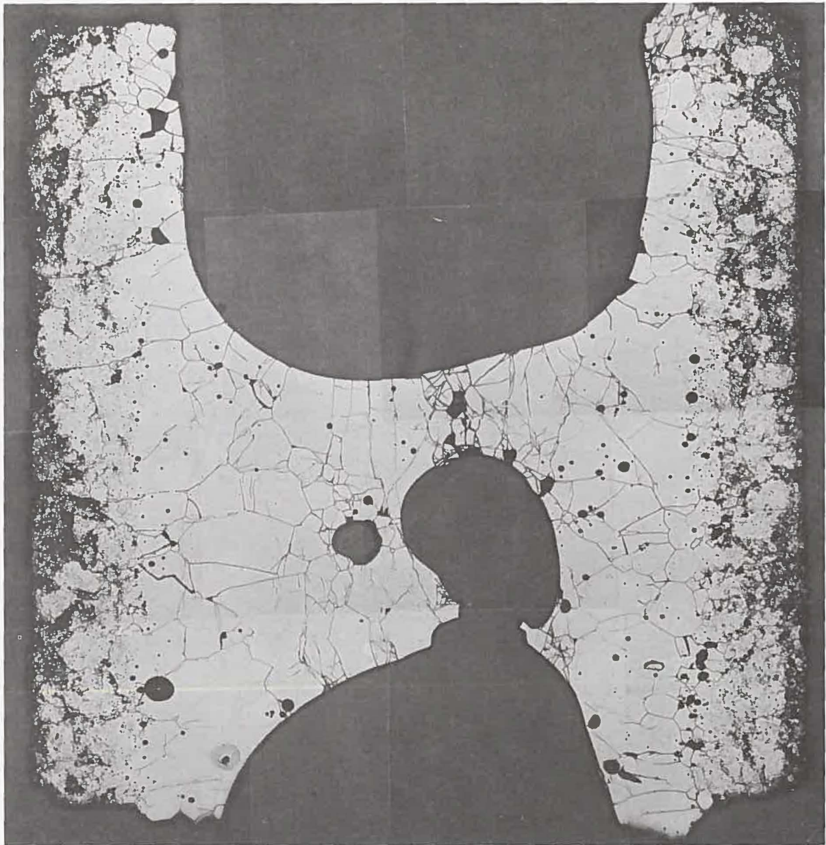
Fig. 76 Longitudinal Section of Fuel Pellet Showing Bridge of Melted Fuel Across Central Void. Neg. No. MSD-186349. ~30X.
