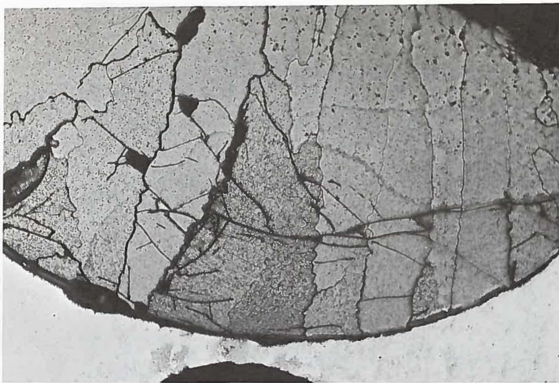
Fig. 51(a) Columnar Grains of Melted Fuel. Neg. No. MSD-185238.
