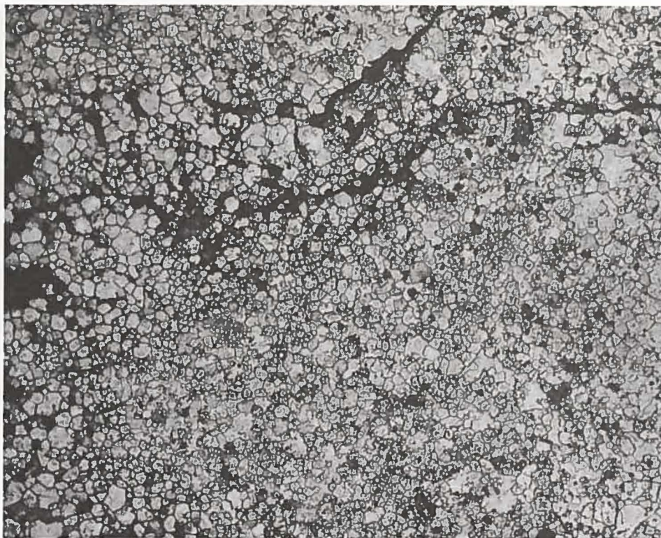
Fig. 50(a) Small Grains in Unmelted Fuel. Neg. No. MSD-185241.
