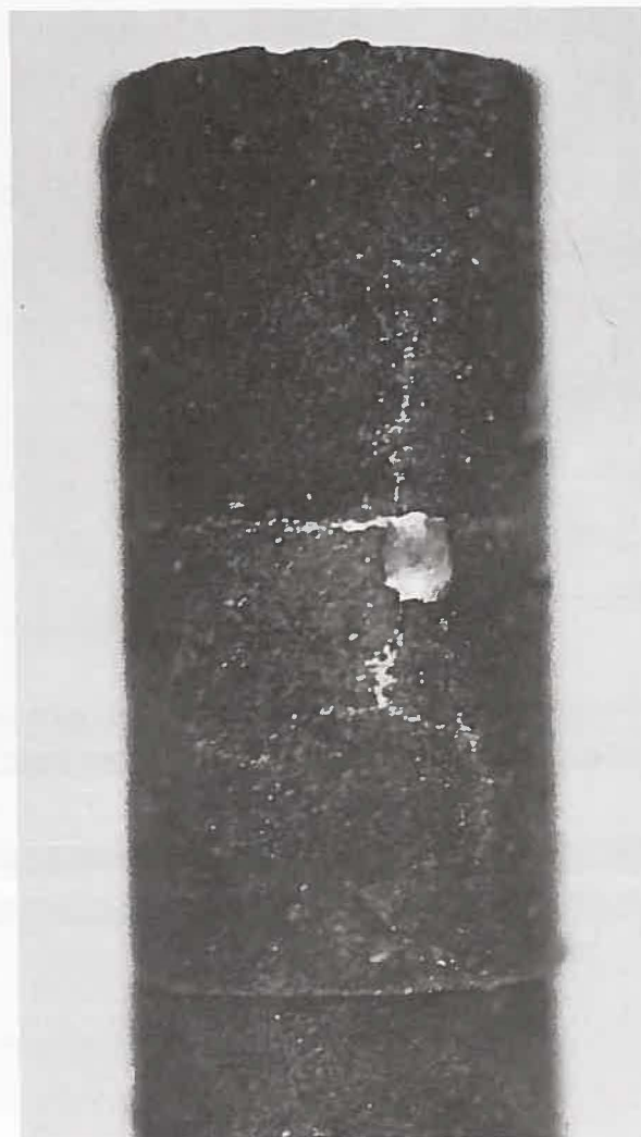
Fig. 85(b) Some Degree of Wetting by Globule of Melted Steel on Fuel Surface. Neg. No. MSD-185670. 11X.
