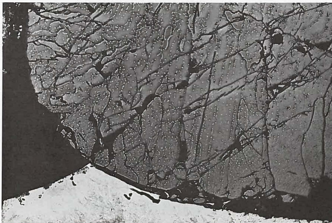
Fig. 51(b) Columnar Grains of Melted Fuel with Globules of Steel. Neg. No. MSD-185239
