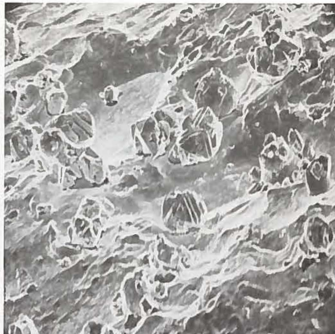
Fig. 52(b). Crystalline Projections on Surface of Central Void. Neg. No. MSD-200552.
