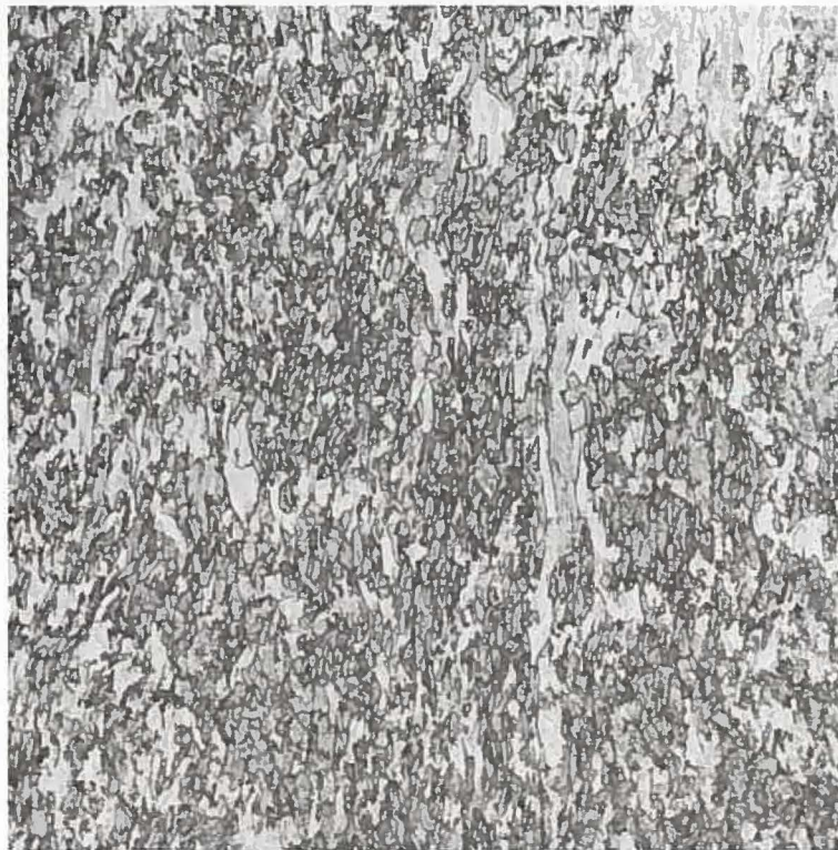
Fig. 66(b). Microstructure of Molybdenum Tube from Top of Section 92-R4-70. Neg. No. MSD-184778. 150X Etched.
