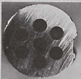
SECTION B. 0.6 CM ABOVE BOTTOM OF FUEL COLUMN. UNMELTED FUEL PELLETS IN MATRIX OF STAINLESS STEEL.
