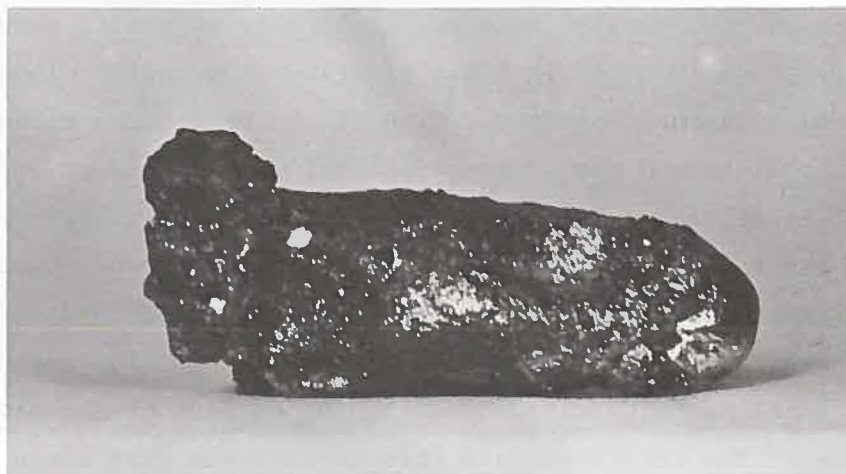
Fig. 53(b) Steel Ingot with Fuel Removed. Neg. No. MSD-183801.
