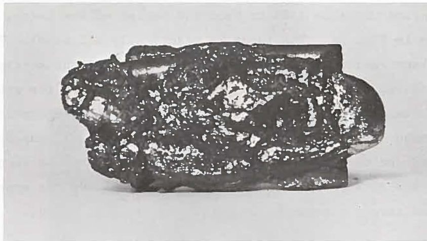
Fig. 53(a) Steel Ingot with Fuel Attached from Upper Part of Section 40-R4-17. Neg. No. MSD-183799.
