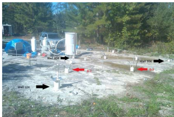
Figure 4: A photograph of the experimental site. The DTS instrument, spa-heater, and storage tank are visible near well 404.
