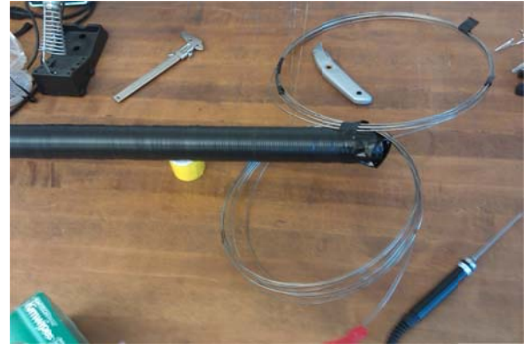
Figure 2: Close up of threaded PVC pipe wrapped with fiber optic cable and secured with electrical tape.
