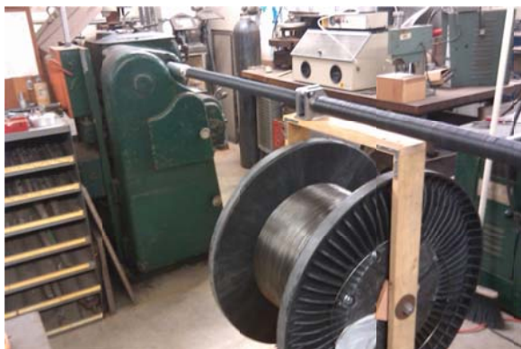
Figure 1: Process of wrapping fiber optic cable around a threaded PVC pipe assisted by a lathe.
