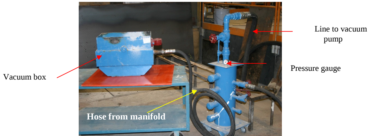
Figure 4.2.1 Vacuum box and pressure manifold system.
