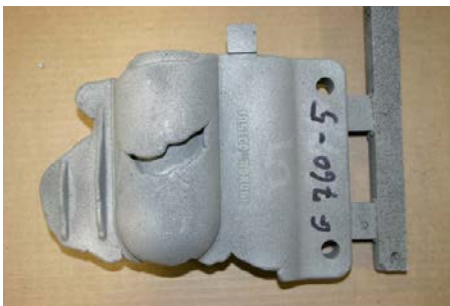
(a) N5181-5c, no vacuum, not filled, misrun.
