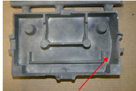
Compaction defect (b) N5181-3c, front.
