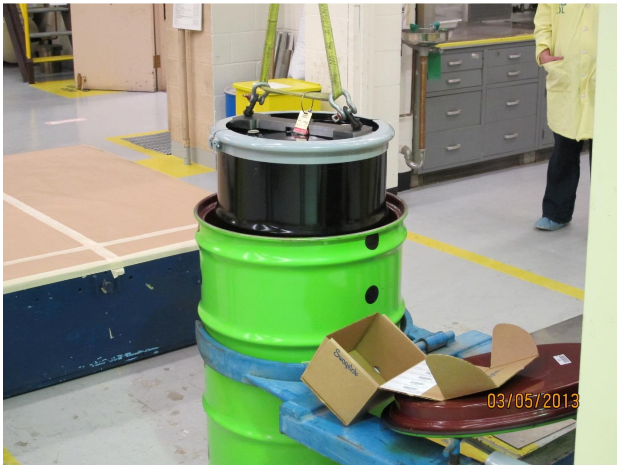
Picture 7. Lifting the inner drum out of the outer 9979 shipping drum.
