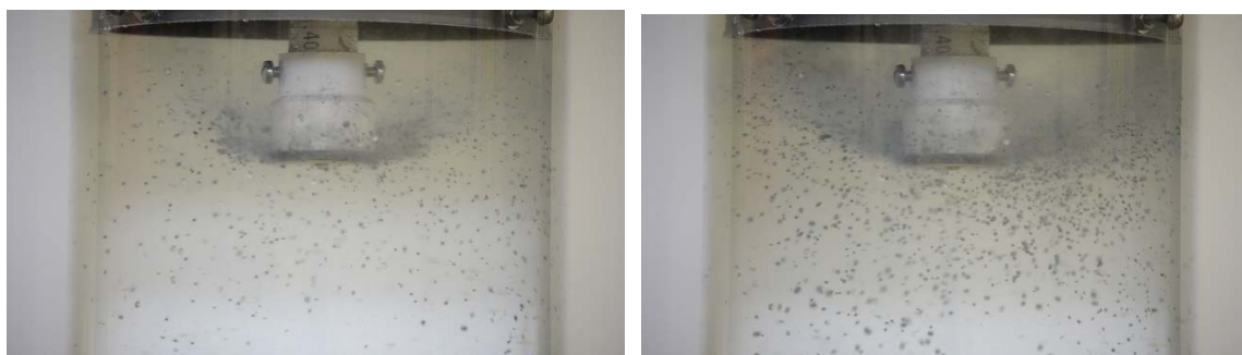
Figure 2-25. Droplets produced with impeller turning at 1100 RPM and 1.75 gpm water flow rate through chamber.
