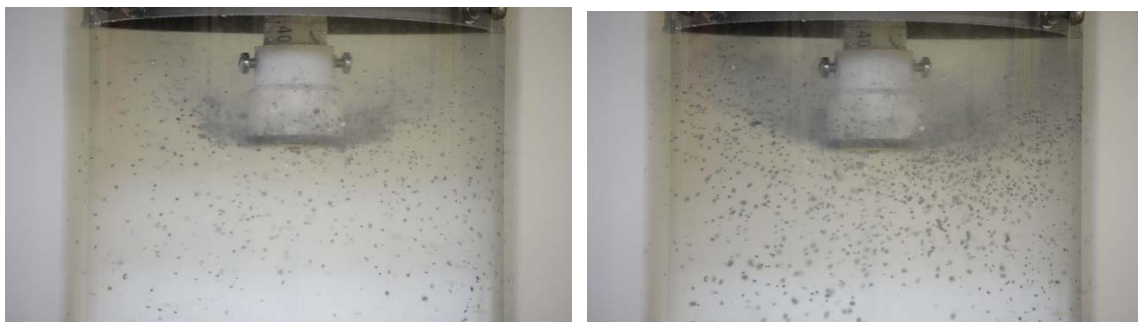
Figure 1-4. Droplets produced with impeller turning at 1100 RPM and 1.75 gpm water flow rate through chamber
