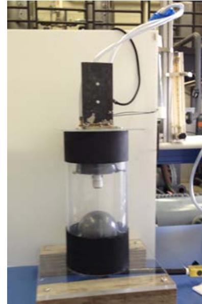
Figure 2-16. Experimental cold-flow combustor simulation apparatus. Left: Diagram at left shows major components. Right: Photo of apparatus configured for tests.
