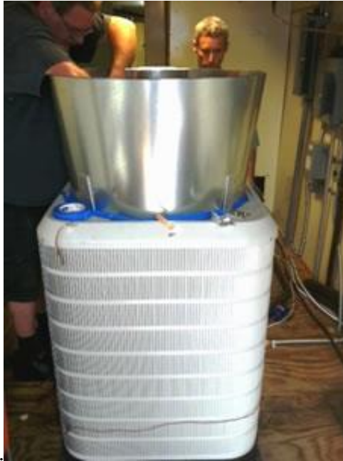
Figure 6. Fabrication of 7-degree divergent diffuser
