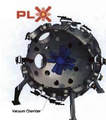
Imploding plasma liner formed by 30 merging plasma jets with 1.5 MJ capacitive stored energy
