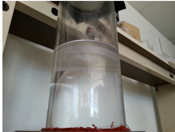
Figure 64. TES Crust Formation in Test Vessel
