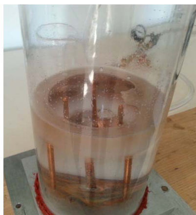
Figure 65. Crust Formation Around Heat Pipes
