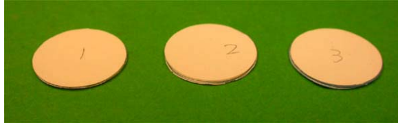
Figure 13: Multilayer specimens of NEB20/DuPont 951 laminated only by isostatic pressing at RT.
