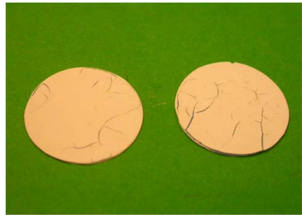
Figure 9: Sandwich specimen of NEB20/DuPont laminated using a uniaxial press followed by CIP and co-firing at 850°C for 0.5 hours.
