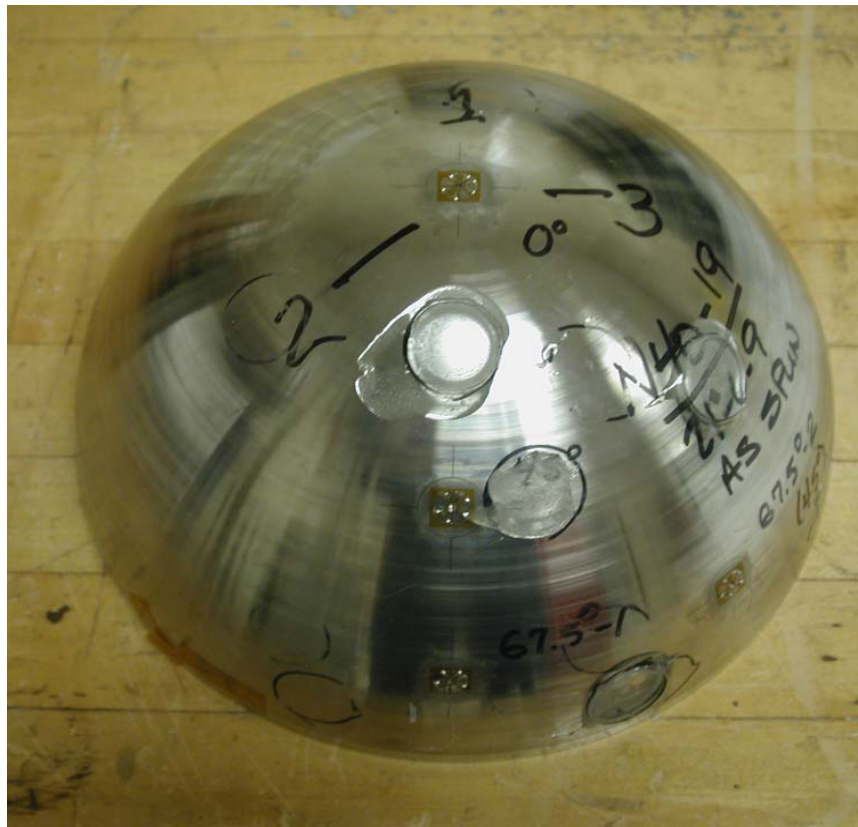
Figure 4 Residual stress test locations after testing. The bronze-colored strain rosettes are visible at 0° (Pole location), 45°, and 67.5° (Near waist). The holes for the test were drilled in the center of each strain rosette. Leftover epoxy is visible where the feet for the drill press had been glued to the hemisphere.
