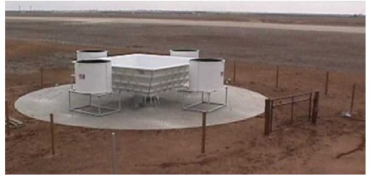
Figure 3-10 (left): Texas Tech 200-m tall tower at Reese Technology Center; (upper right): lowest three levels of instrumentation on the 200 m tower showing the various instrumentation on each boom arm; (lower right): TTU Vaisala LAP-3000 Boundary Layer Profiler
