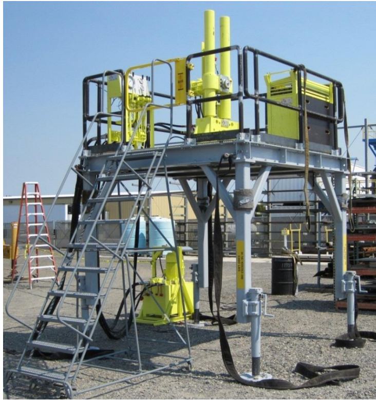
Figure 2-2. Cone Penetrometer Equipment on the Test Platform
