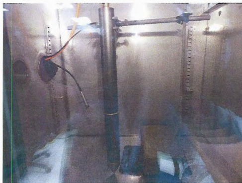
Figure 1. Cone Penetrometer Load Cell in Environmental Chamber.
