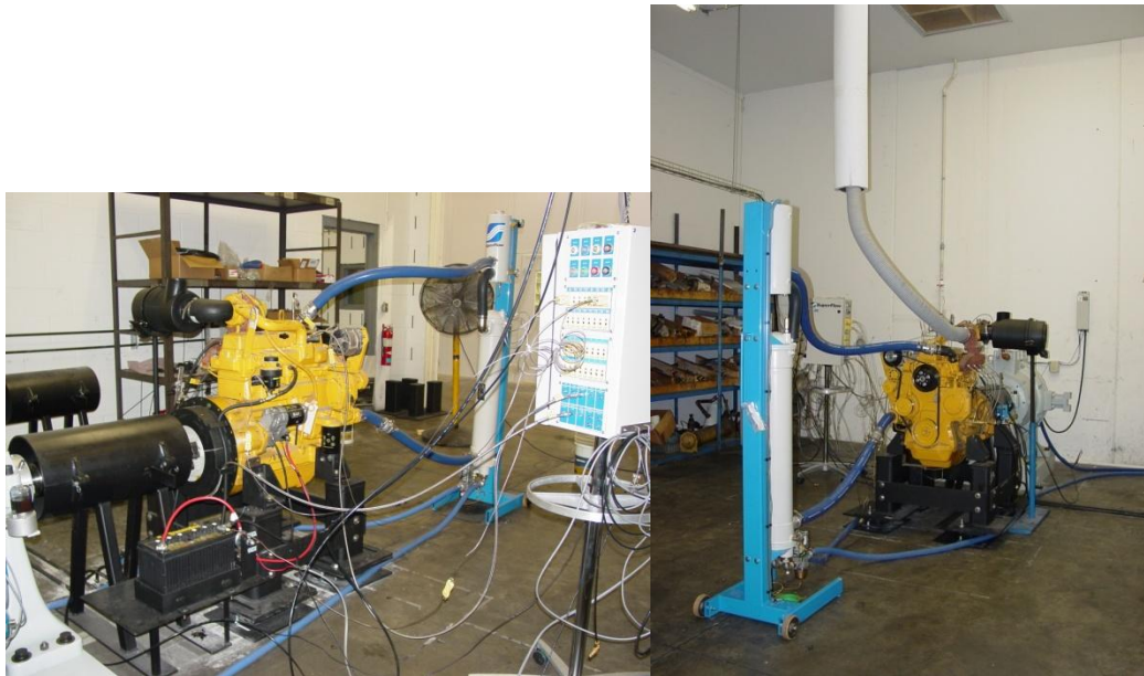
Figure 2: 120 HP John Deere Diesel Engine
