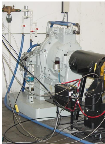
Figure 3: 300 HP Eddy Current Dynamotor
