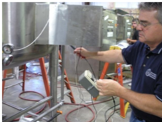
Figure 7: Microwave Leak Detector
