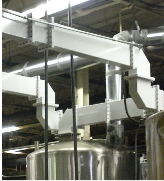
Figure 3: An 800-Gallon Stainless Steel Grease Reactor
