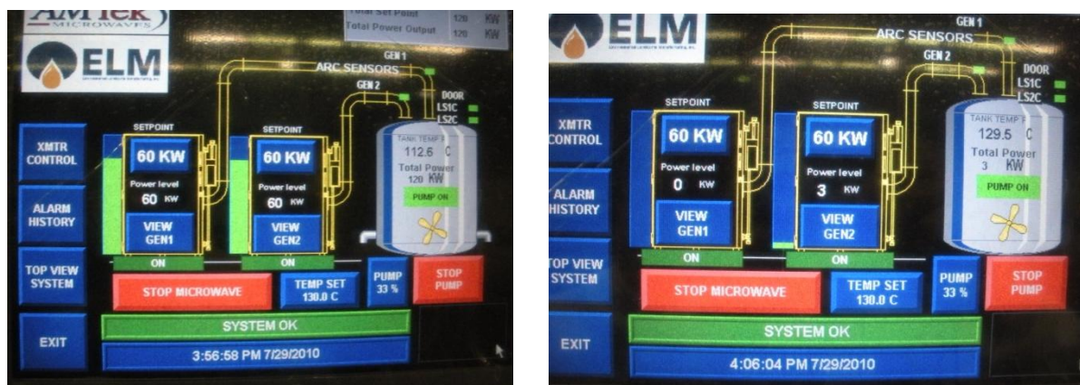
Figure 4A: The set temperature is 130 °C transmitters are at 60 kW each. Figure 4B: tank temperature is 129.5 °C and the controller has automatically adjusted the transmitters to 0 kW and 3 kW.
