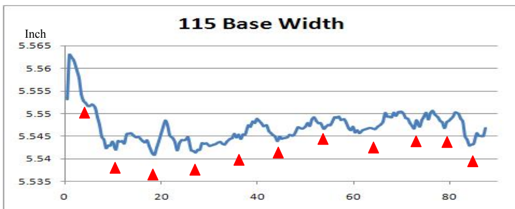
Figure 7. A sample flange width measurements along a 115RE rail. (Red triangles indicating the cyclic dips)
