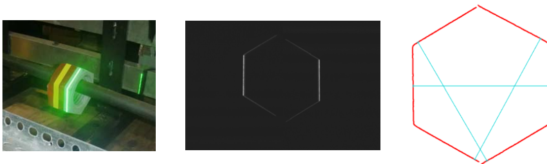
Figure 2. Calibration using a hexagon master piece. (Left) The hexagon set up in position, illuminated by laser lines (Middle) Images of the hexagon taken by two cameras (Right) Constructed hexagon profile after calibration
