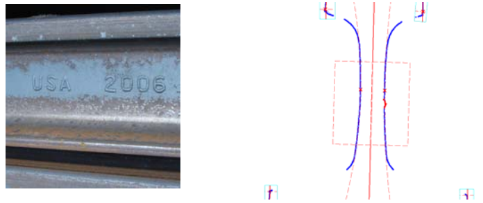
Figure 10. Print on the rail web and the detection with the in-line metrology
