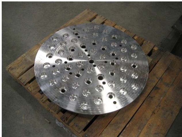
Figure 110. Bottom surface of the bottom plate
