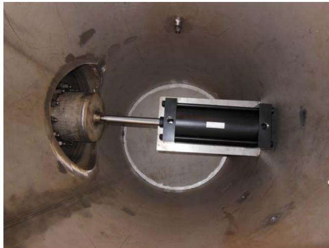
Figure 117. Air piston extended in containment vessel
