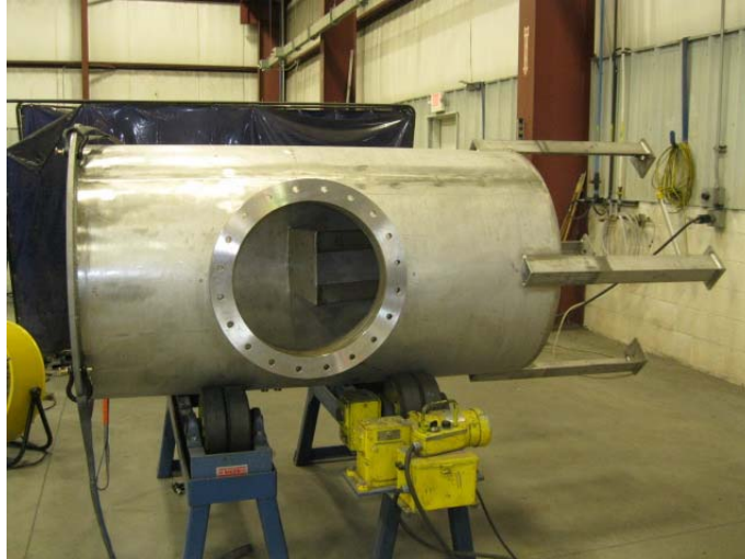
Figure 111. Front view of containment vessel (Note: Vessel is on its side. It's designed to stand on its legs.)
