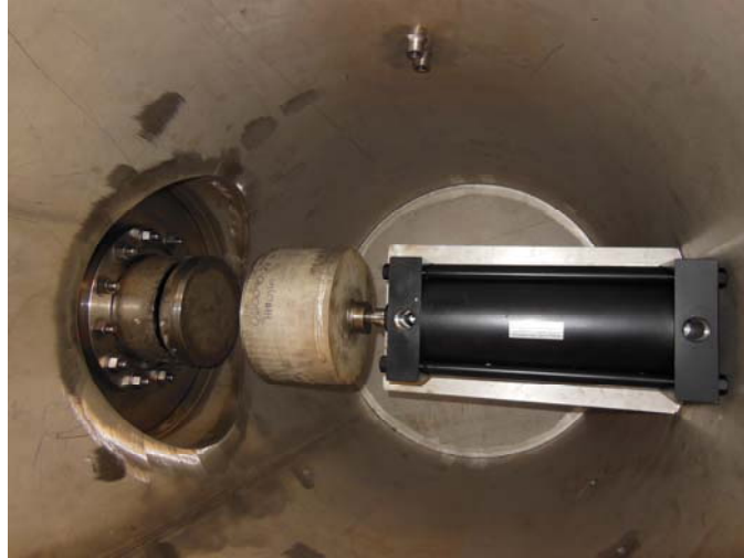
Figure 118. Air piston retracted from circumferential break top hat break plate
