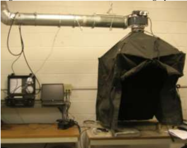
Figure 3: Portable Emissions Monitoring System (PEMS)
