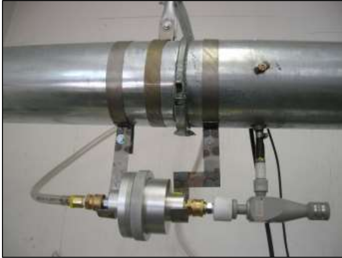
Figure 2: New Gravimetric Pump and Filter System
