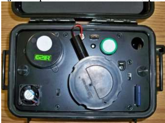
Figure 4: Improved IAP Meter with Wireless Capability
