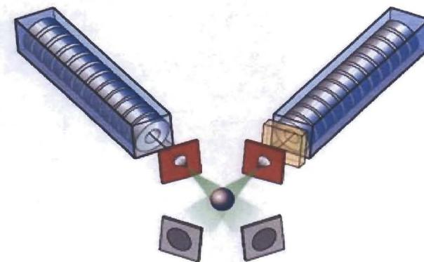
• DARHT: Produces two simultaneous x-ray images. X-ray flashes (the green rays) will be generated when high-energy electron pulses from each accelerator slam into tungsten targets (red).
