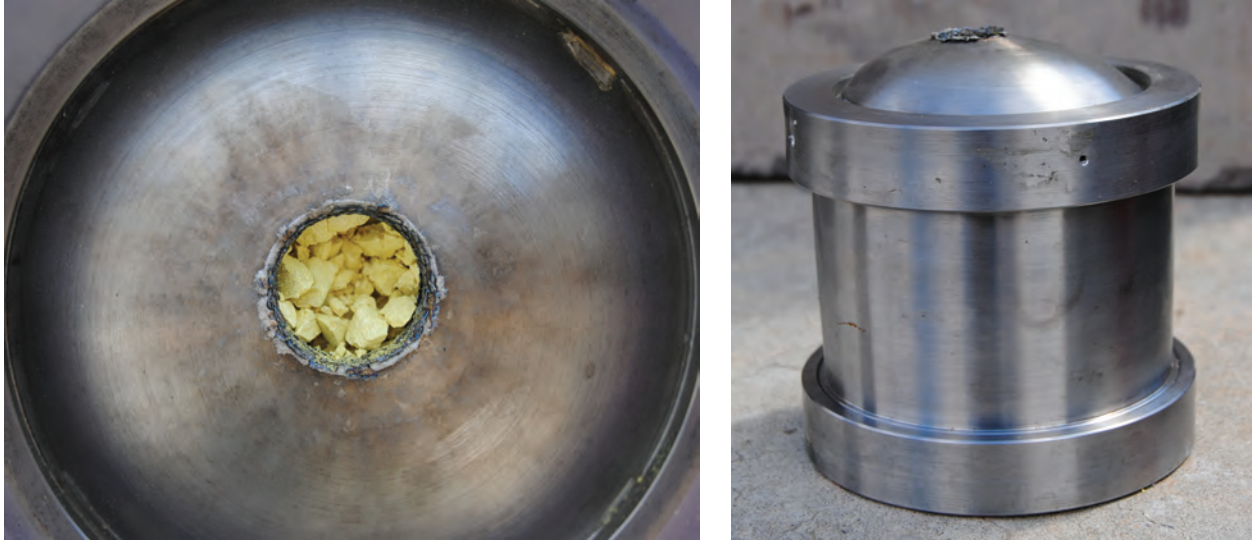
Figure 9: Post-shot photographs of K12-21556. The front plate has bulged considerably, and PBX-9502 fragments are visible through the entry hole. The cylinder wall has also bulged in the impact.
