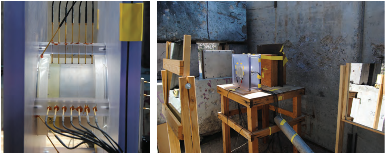
Figure 6: Pre-shot photographs of K12-21570. On the left is a side view of the target cylinder. On the right is a view of the target assembly, x-ray phosphor cassette, and two turning mirrors for the high-speed camera.
