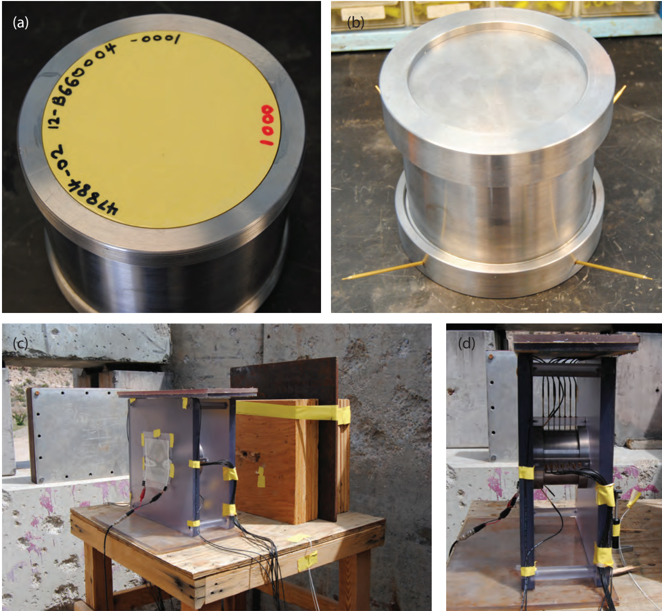
Figure 4: Pre-shot images for K12-21556. (a) The PBX-9502 cylinder in the steel cylinder. The threads used to attach the retaining rings are visible. (b) The back plate of the target. The four front-plate pins are mounted through the front retaining ring. (c) The target assembly in position. MS3 is covering the view of the front of the target. The x-ray cassette holder is in position to the left, and the projectile back stop is to the right of the target. (d) Side view of the target assembly showing pin rails. The PDV probe mounting hardware and fibers are visible to the left.
