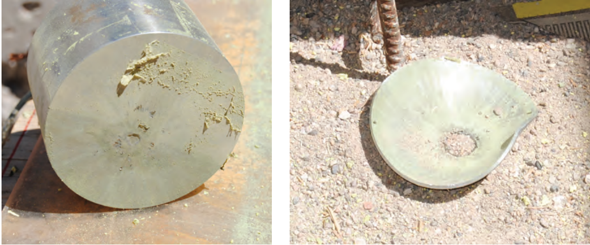
Figure 17: Post-shot photographs of the steel cylinder (left) and front plate (right). A small dent is visible on the face of the steel cylinder, though it is not deep.
