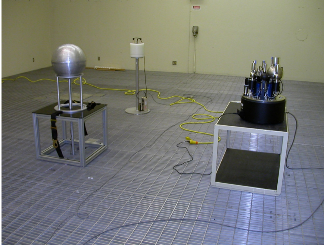
Figure 9. Neutron spectra and dose rates measurements with ROSPEC and SWENDI-II (dose rates only) with D 2 O moderated 252 Cf source
