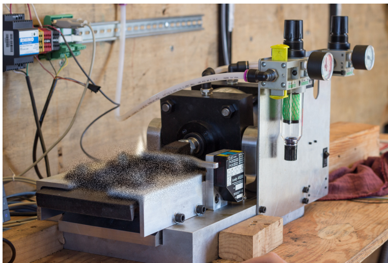
Figure 6: Articulation fatigue test rig for 500 kW-scale “v3” belt attachment system.
