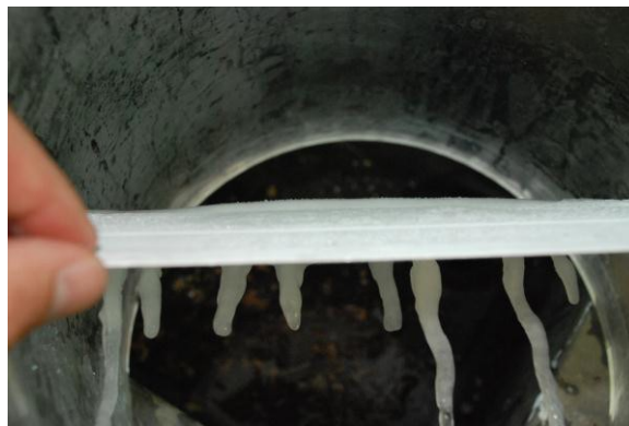
Figure 19. Trailing Edge View Ice Formation on Airfoil Treated with CRC6040R3
