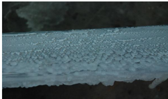
Figure 22. After Icing Test Results – Zoomed in View of Upper Surface
