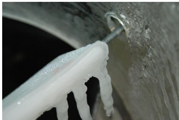
Figure 20. Side View of Leading Edge Ice Formation on Airfoil Treated with CRC6040R3
