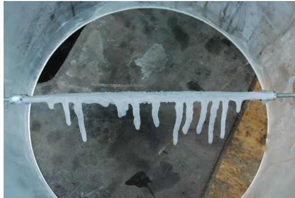
Figure 21. Leading Edge Ice Formation on Airfoil Treated with PhaseBreak TP
