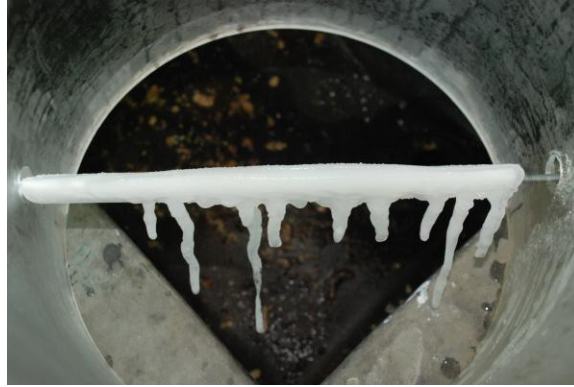
Figure 18. Leading Edge Ice Formation on Airfoil Treated with CRC6040R3
