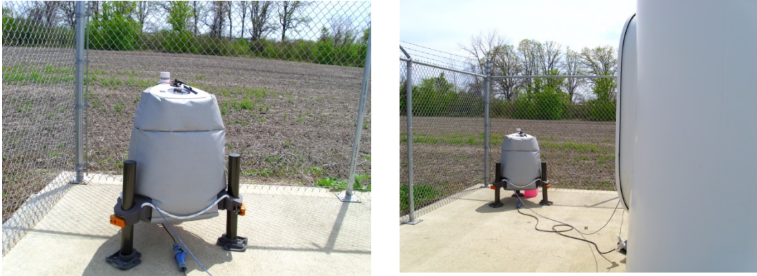
Figure 8. ZephIR 300 LiDAR installed beside the wind turbine tower base at Woodlands School in Huron, Ohio
