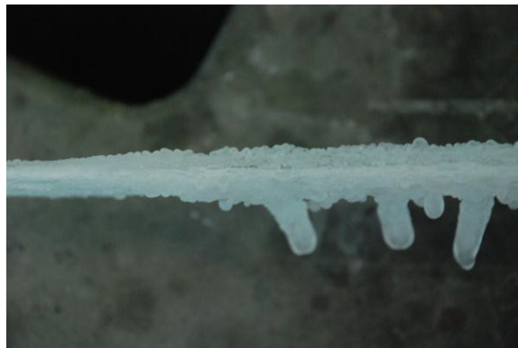
Figure 23. Leading Edge Ice Formation on Airfoil Treated with PhaseBreak ESL
