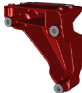
Figure 130: LBD Front Engine Mount
