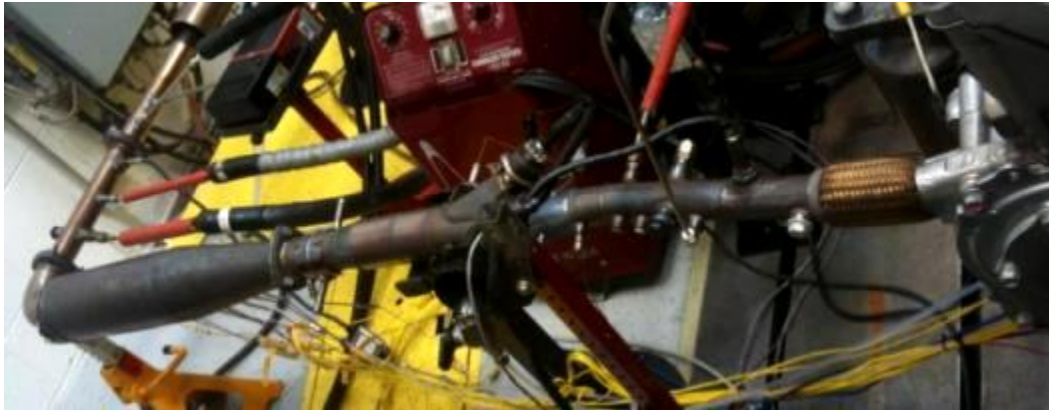
Figure 75: Active Urea Lean Aftertreatment Hardware
