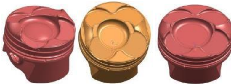
Figure 120: LDB Piston Bowl at Various Bowl Geometries
