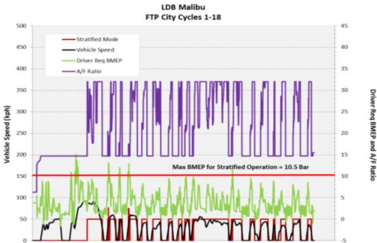
Figure 161: LDB FTP City Lean-Stratified Operation
