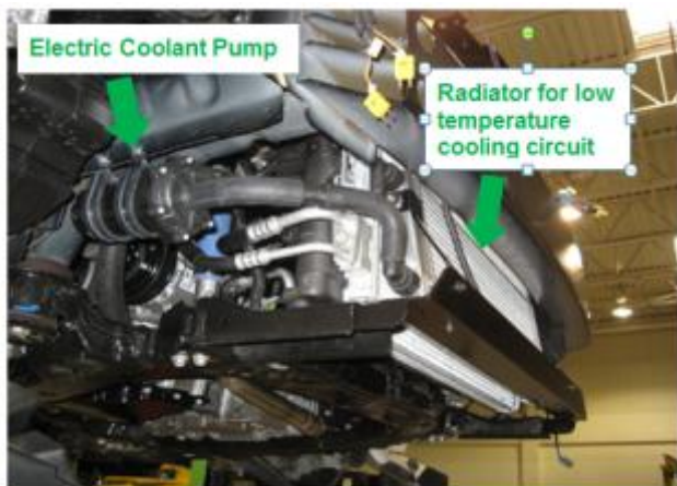
Figure 154: Low Temp Radiator & Aux. Pump
