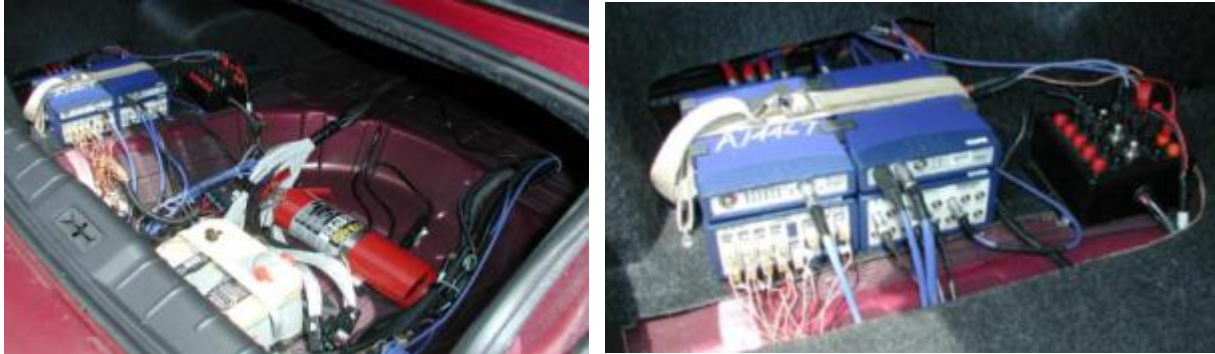
Figure 98: Instrumentation Installation and ETAS Interface Modules
