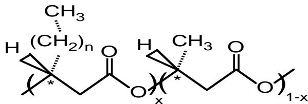
**Figure 1:** Chemical structure of polyhydroxyalkanoates (PHAs) investigated. PHB is poly (3-hydroxybutyric acid) (x=0), PHBV is poly (3-hydroxybutyric acid-*co*-3-hydroxyvaleric acid) (n=1) and PHBHx is poly (3-hydroxybutyric acid-*co*-3-hydroxyhexanoic acid) (n=2). HB, HV and HHx have methyl, ethyl and propyl side chains respectively. The value of x (mcl-3HA units) is between 2 to 50 %.
