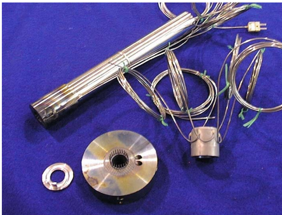
Figure 3. Photograph of Subscale Catalytic Reactor Components for Hydrogen Combustion
