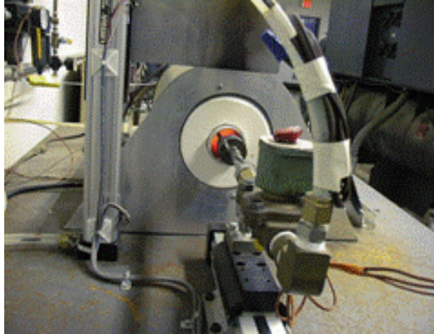
Figure 27. Thermal Cycling Test Rig
