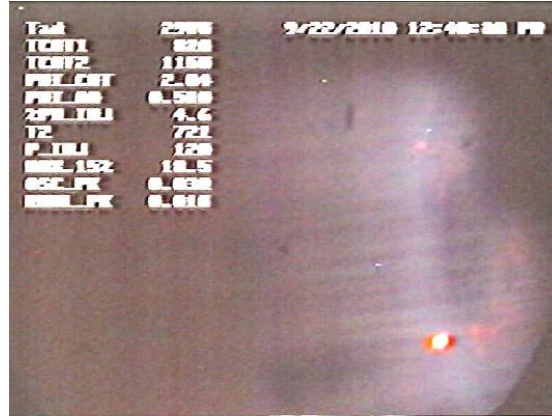
Figure 22. Hydrogen Flame Picture Doped with Natural Gas at Pressure of 8 atm.
