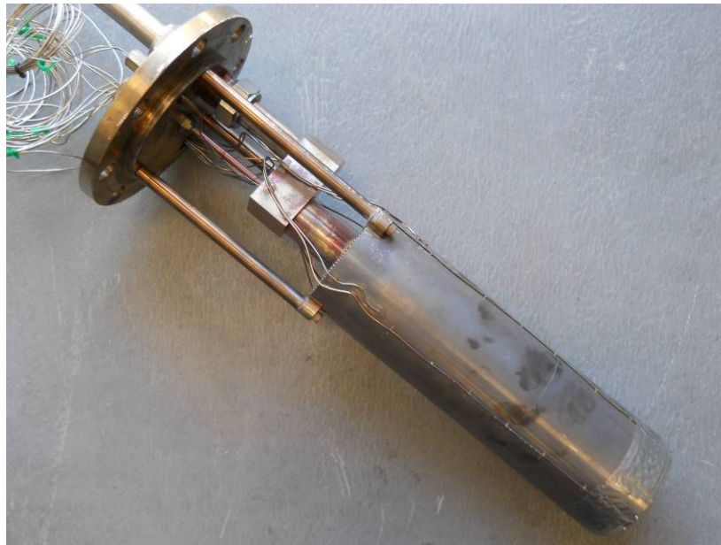
Figure 23. RCH1 Hardware after Testing Showing Good Integrity and Robustness
