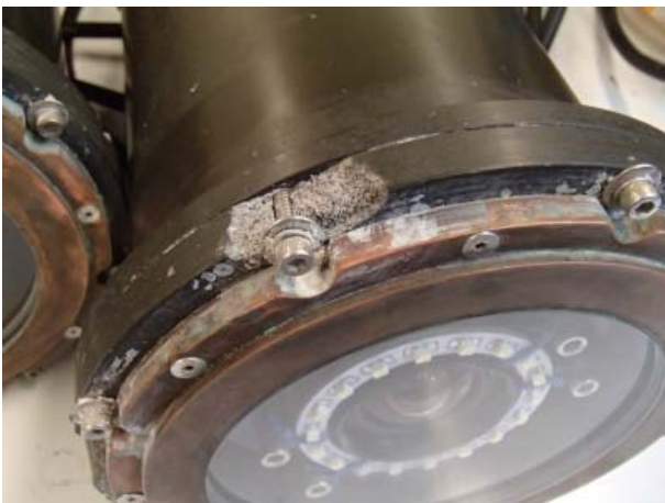
(a) Corrosion on a camera optical port end cap
