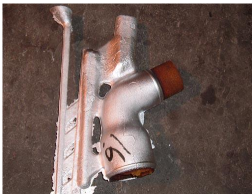
(a) Casting with gating system and core.
