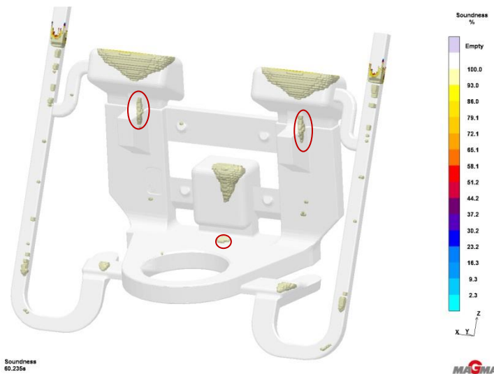
Figure 4.5.21 Minor secondary shrinkage predicted underneath top risers.
