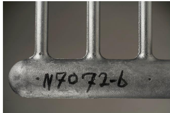
(b) N7072-6, 445°C, 0.043%Ti, no hot tear.
