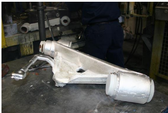
(a) Casting with sand core and test bar prolongation
