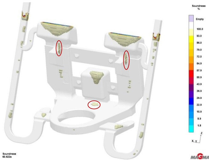
Figure 4.5.24 Areas where minor shrinkage is predicted when die opens.
