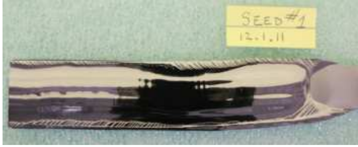
Figure 7 Picture of single-crystal ribbon growth. Left side is a (111) facet.
