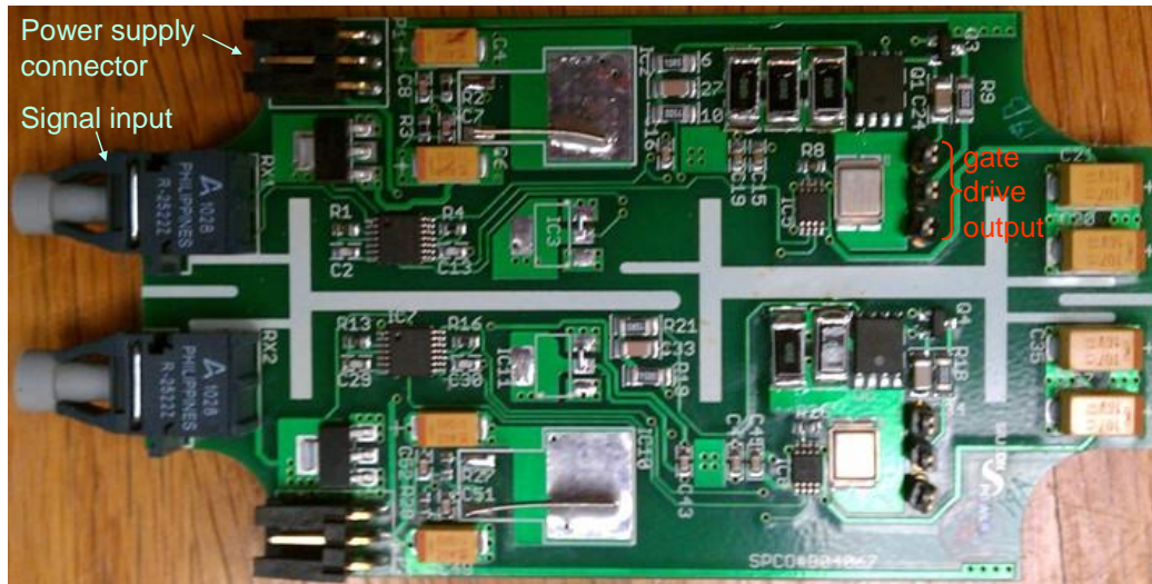
Figure 7-4. Gate driver board that fits the module footprint.
