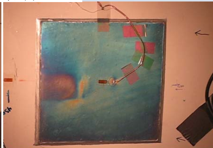
Shot at minimum load: minimum compression load on lower surface, minimum tensile load on upper surface.
