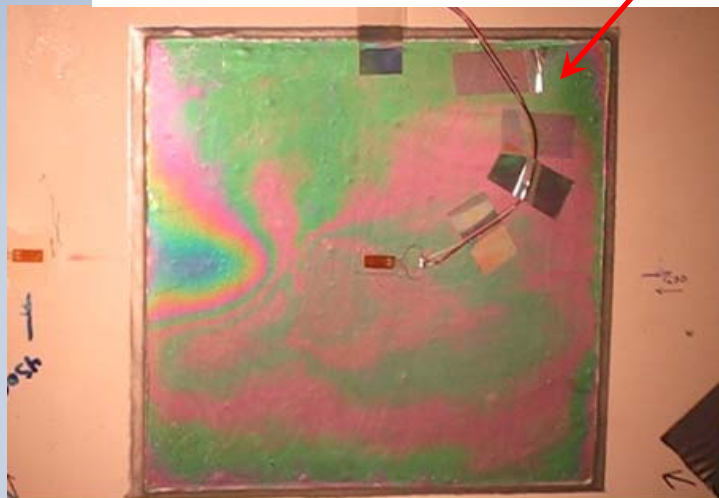
Shot at maximum load: maximum compression load on lower surface, maximum tensile load on upper surface.
